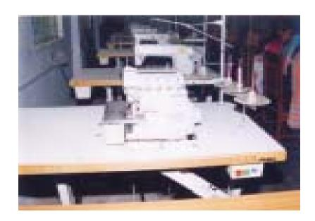
**OVERLOCK MACHINE-3 THREADS**
